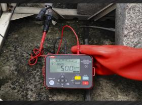
After measurement, the output voltage is turned off, the Tester discharges electricity automatically at a fast speed, and the LCD holds the present measurement information and data.
